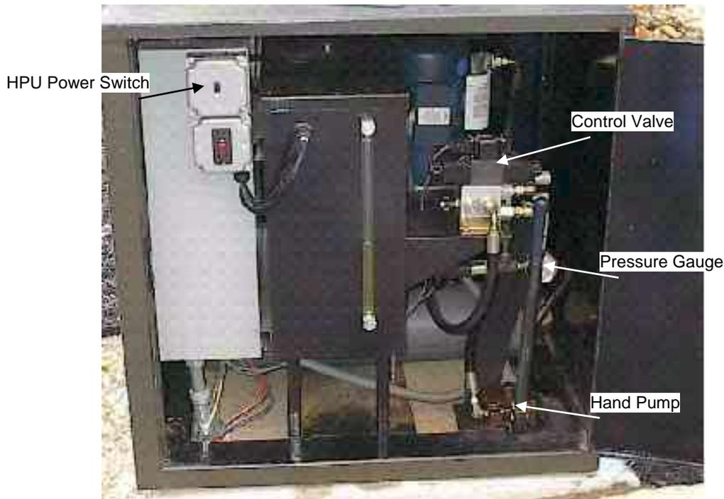
**Figure 2 Model 6119 HPU without EFO Manifold**
