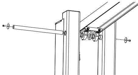
3. Lock shaft in place using locking screws in each bearing and shaft lock washers on either side of drive stanchion.
